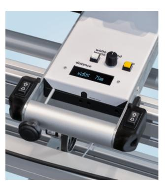
Innovative control panel for speed and drive direction. Digital Display shows length and width measurements.
